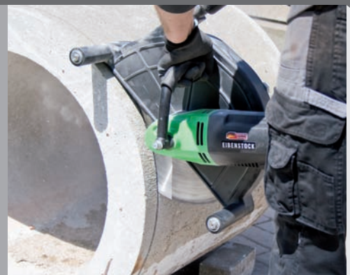
Working near to the edge with accessory set + diamond cutting disc (accessory)
